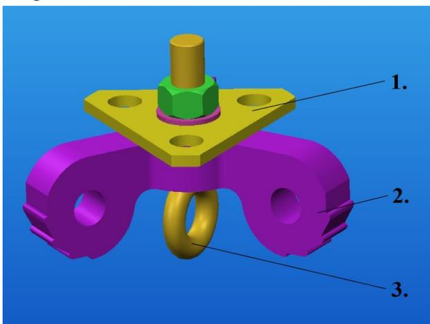
Figure 2. Connection subassembly (1-anchor flange, 2-fixing body, 3-retaining ring).
