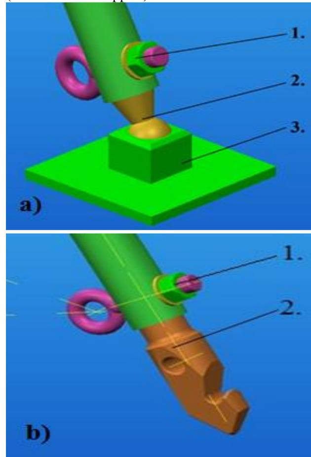
Figure 5. Fixing system, on the ground: a) sole plate (1- bolt, 2-ball joint, 3-sole plate), b) claw fixing (1- bolt, 2- claw);
