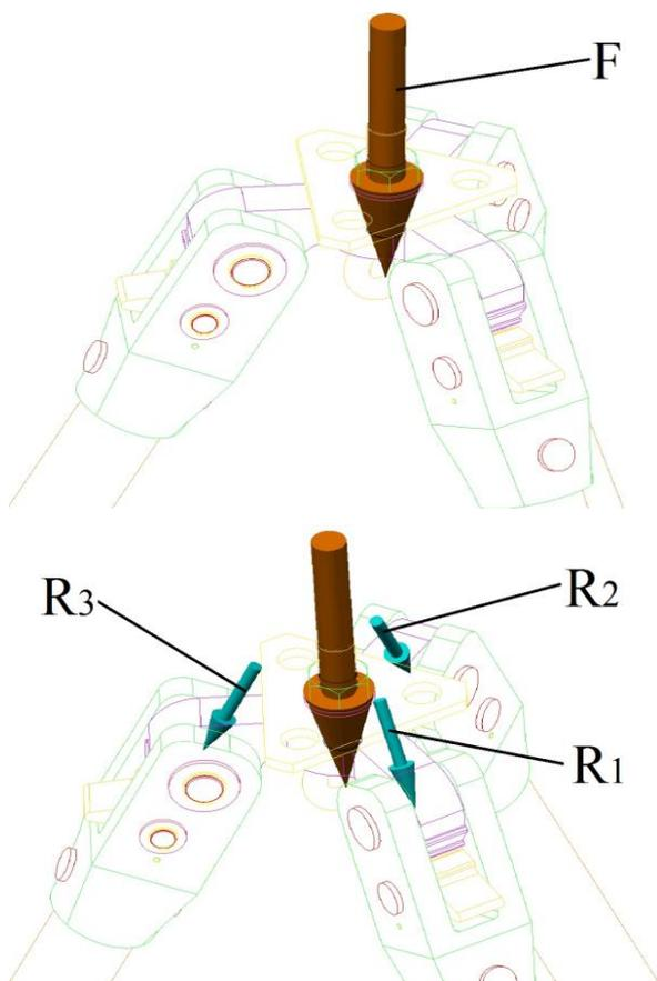
Figure 6. a) Forces on to the tripod, b) Force components;
