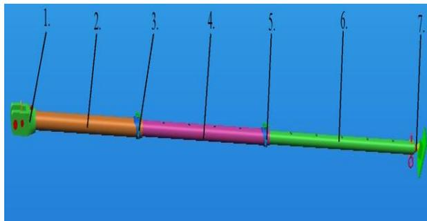
Figure 3. Support subassembly; (1- cylindrical hinge, 2, 4, 6 –telescopic legs (sections), 3, 5- locking sections system, 7- support and anchoring system).
