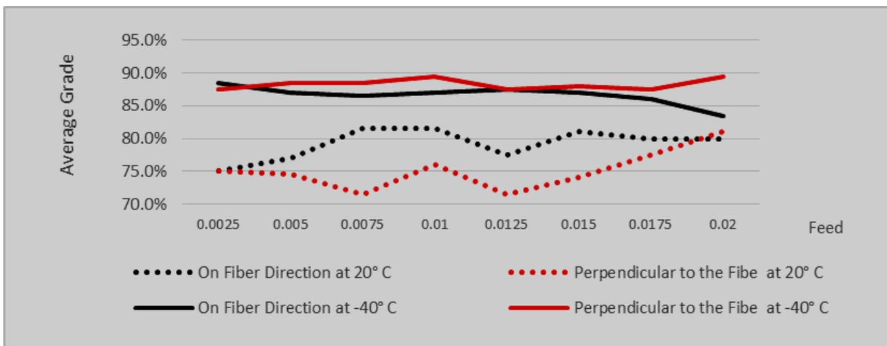
Figure 4. Evolution of the quality at milling vulcanized rubber with the cutting speed 3297 m/min, at the material 3540, depending on the feed
