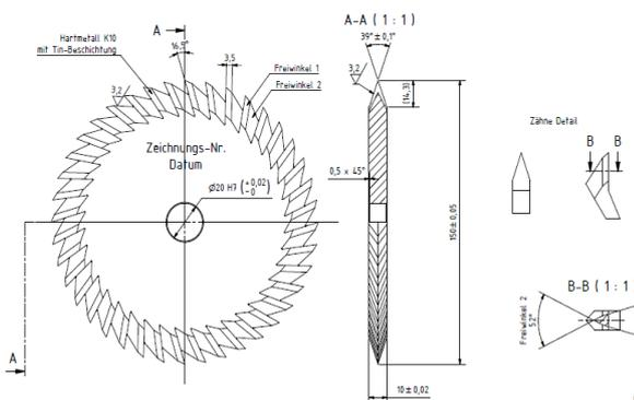
Figure 2. Tool used in experiment
