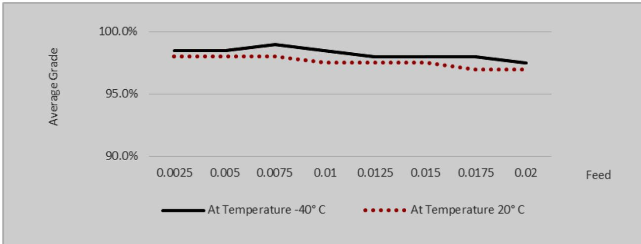
**Figure 5. Evolution of the quality at milling vulcanized rubber with the cutting speed 3297 m/min, at the material 3003, depending on the feed**
