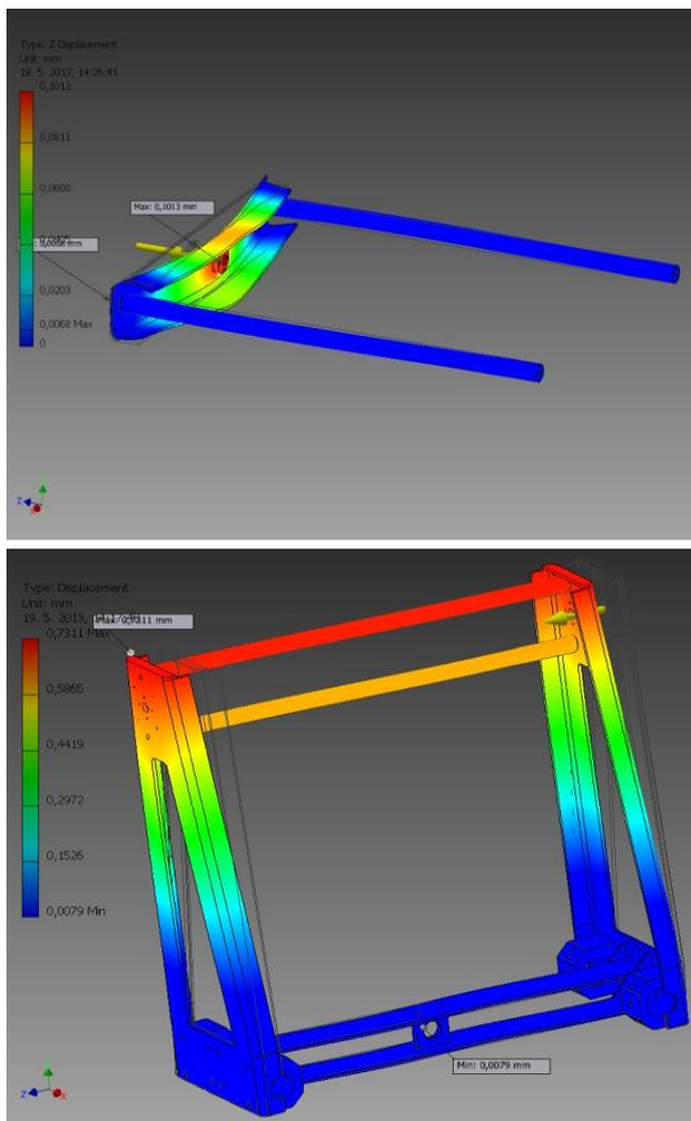
**Figure 3. Static analysis of device parts in Autodesk Inventor Professional 2013**
