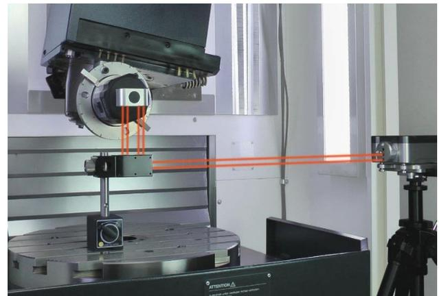
**Figure 6. Measuring rotary axis with Renishaw Ballbar XL-80**
