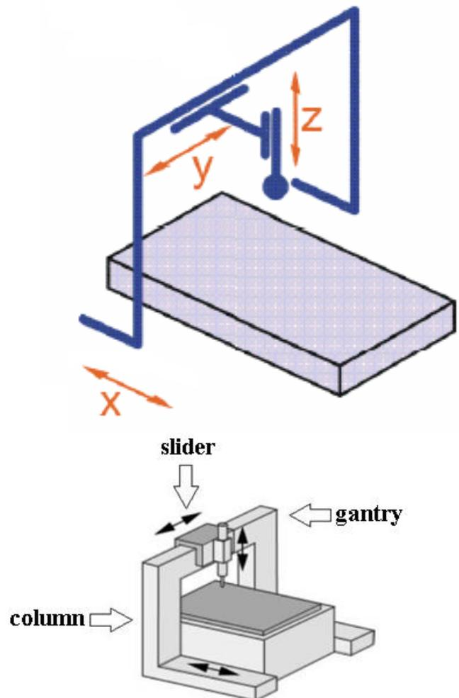
Figure 2. Kinematic scheme of device
