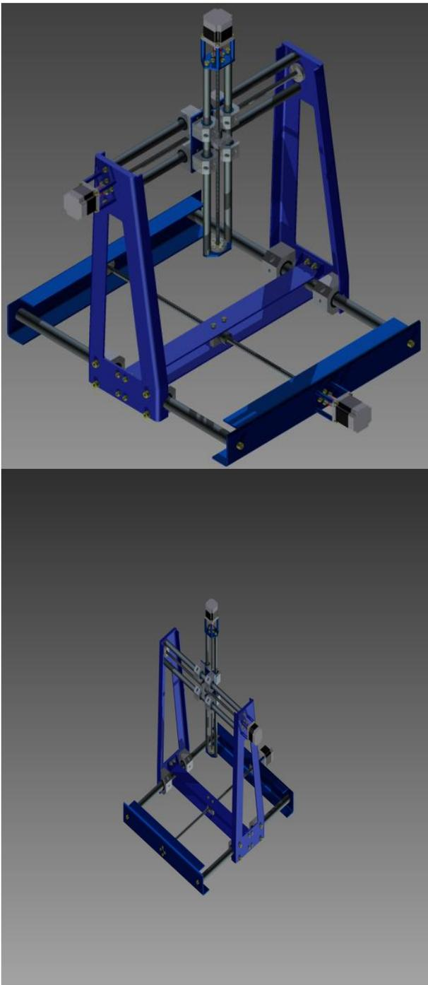
Figure 1. Model of experimental device for practicing routines of machine tool precision measurement
