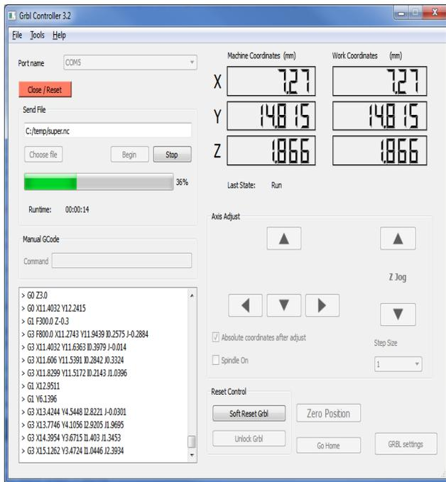
Figure 4. Standard user interface of Grbl controlling software
