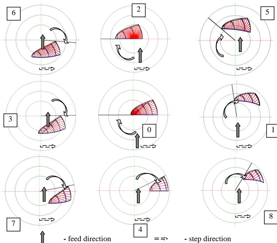
Figure 5. Tool radius projection and uncut chip positions in 5-axes machining
