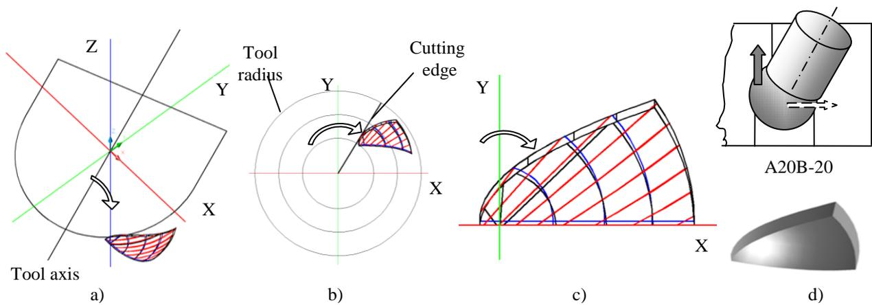
Figure 4. Example of CAD study for A20B-20 tilting tool position
