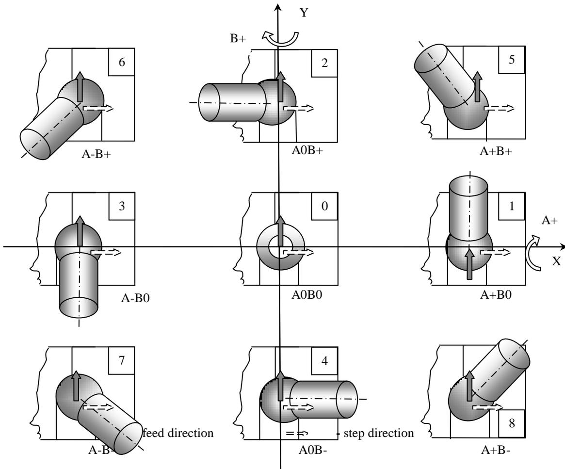
Figure 3. Tilted tool relative position in five-axes machining
