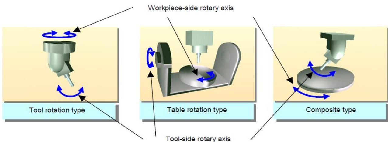
Figure 2. Different types of five-axes machines
