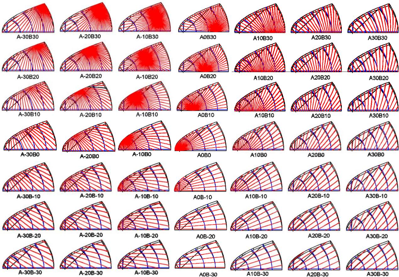
Figure 6. Chips and cross sections in 3D-CAD projection in 5-axes machining
