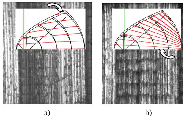
Figure 8. Surface appearance at opposite entrances (fig. a) good and fig b) worse)
