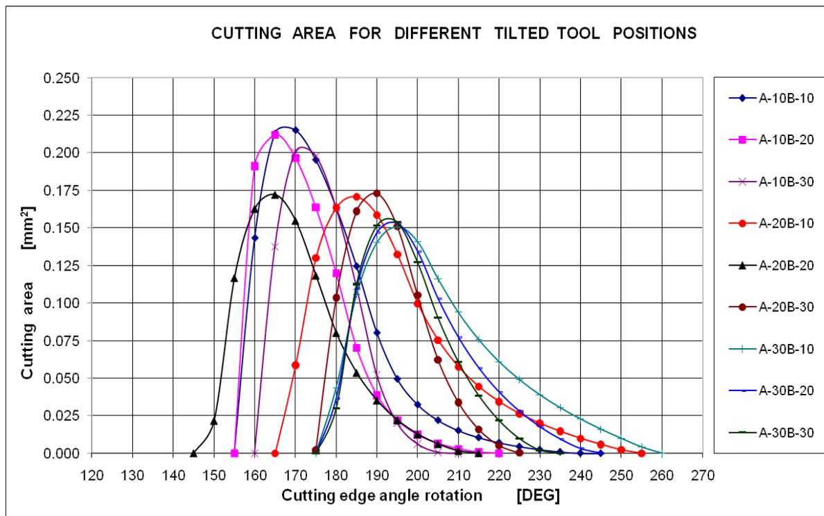
Figure 9. Cutting area for the best entrance of cutting edge
