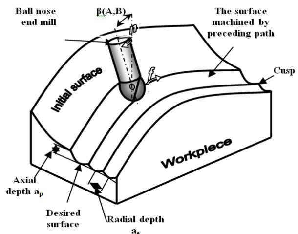
Figure 1. Tool path orientations
