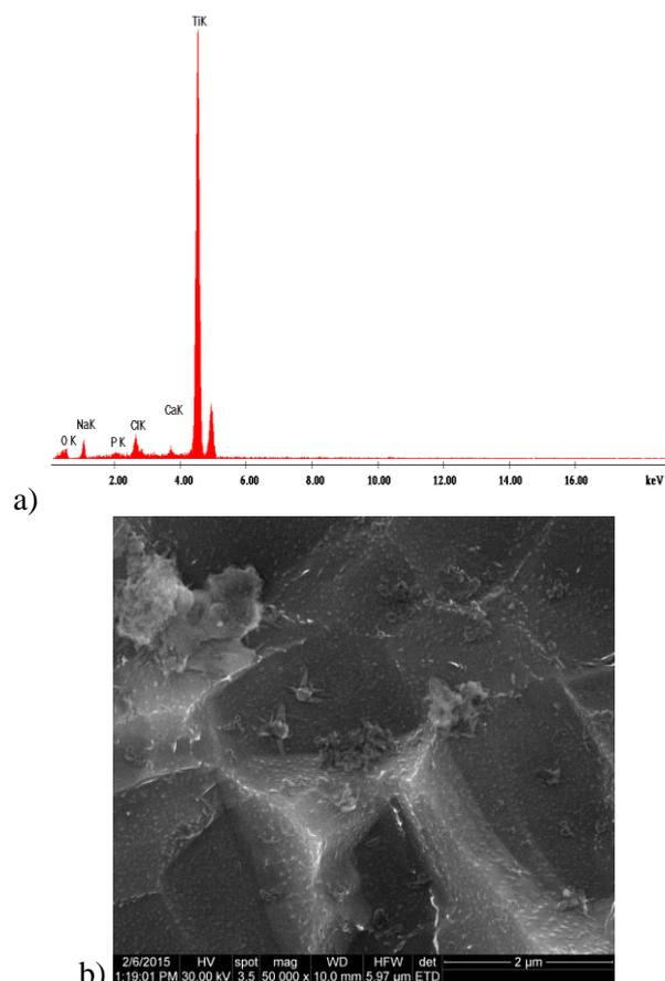
**Figure 2. a) EDX spectrum of M<sub>1</sub> implant after biomimetic coating with  $\beta$ -TCP and Chitosan for 48h, b) SEM image of biomimetic coating at 50,000x magnification**
