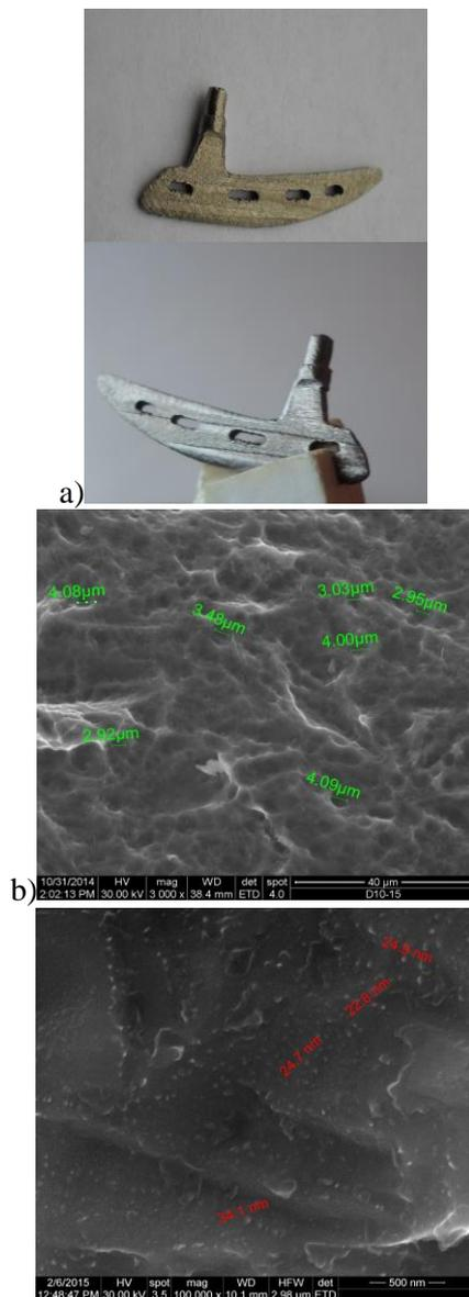
**Figure 3. a) Blade implants  $M_3$ , b) SEM image of  $M_3$  implant surface after acid etching and abrasive blasting, 3000x and 100,000x magnification**
