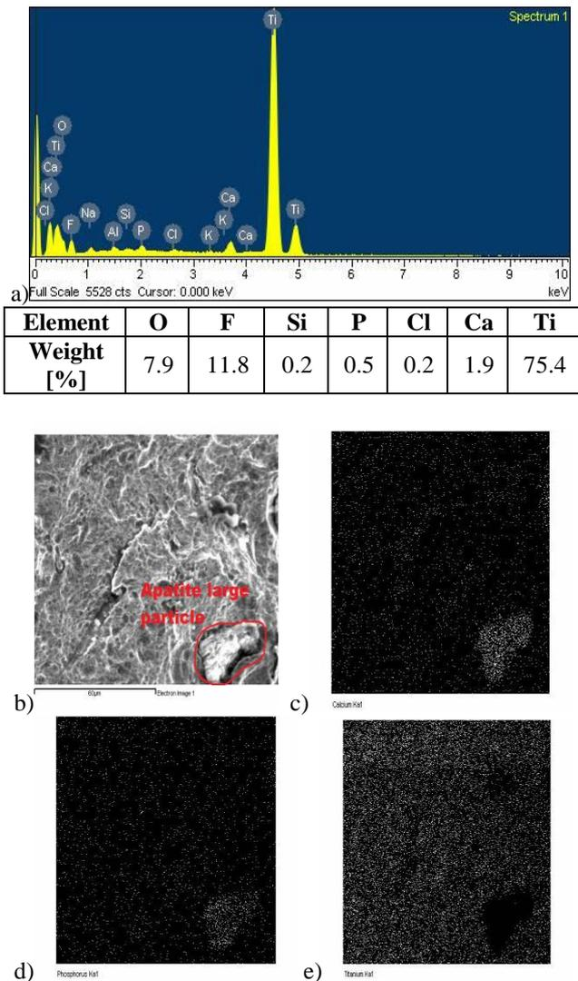
**Figure 4. a) EDS spectrum and chemical composition of M<sub>3</sub> implant after acid etching and abrasive blasting b) SEM image with large apatite particle on M<sub>3</sub> implant surface (1000x magnification), and elemental maps with spatial distribution of c) Ca, d) P and e) Ti**
