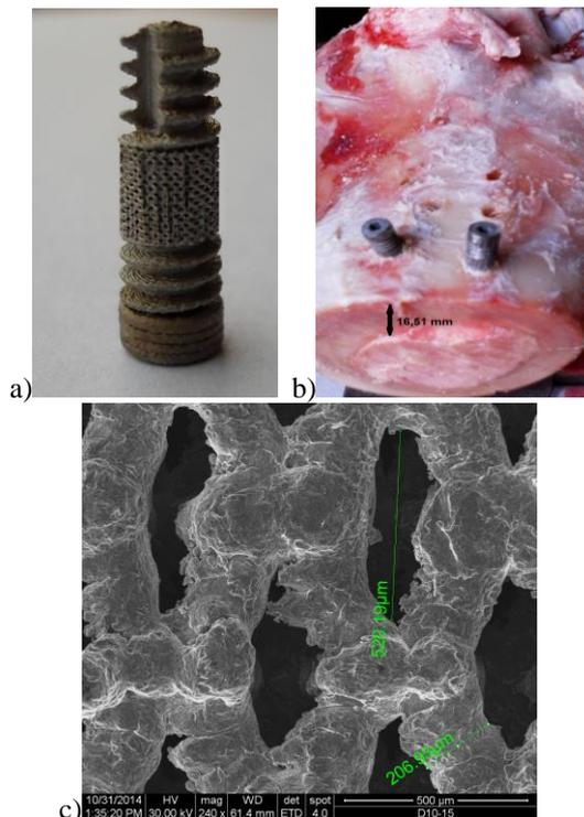
**Figure. 1** Screw vent dental implant: a)  $M_1$  implant after SLM manufacturing, b)  $M_1$  implants during RTT into bovine femur bone, c) SEM image of macroporous structure (cord-support) of  $M_1$ , 240x magnification
