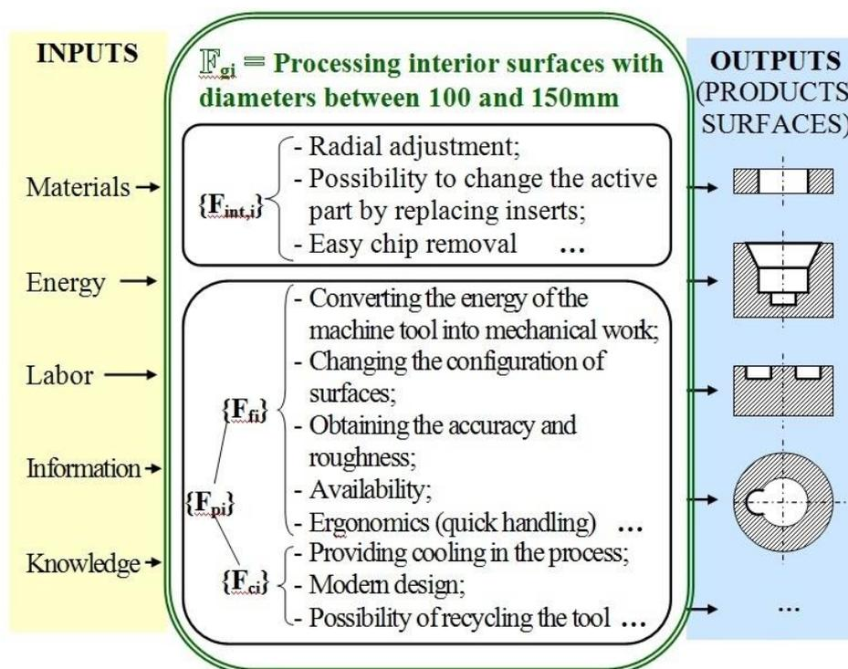
Figure 2. The global function of the boring head model “i”
