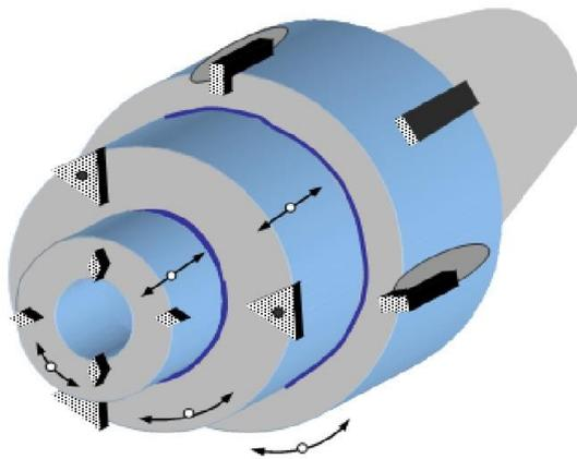
Figure 1. Boring head model “i” with z tangential and radial inserts
