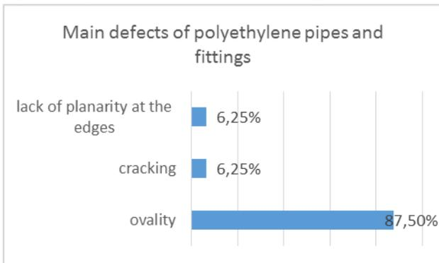
**Figure 8. Main defects of polyethylene pipes and fittings**
