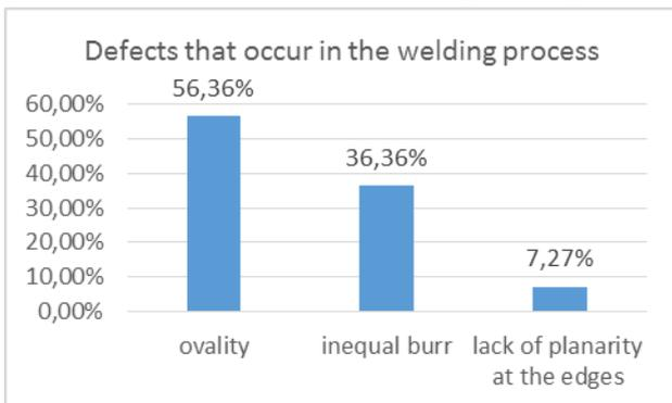
**Figure 9. Defects that occur in the welding process**
