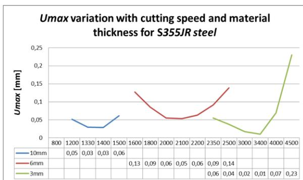
Figure 5.  $U_{max}$  variation with feed rate and material thickness
