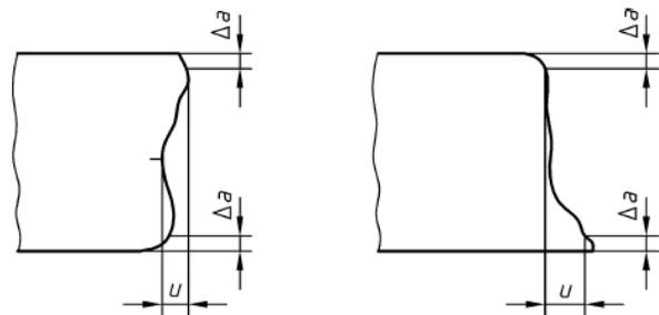
**Figure 1 Perpendicularity or angularity tolerance**
