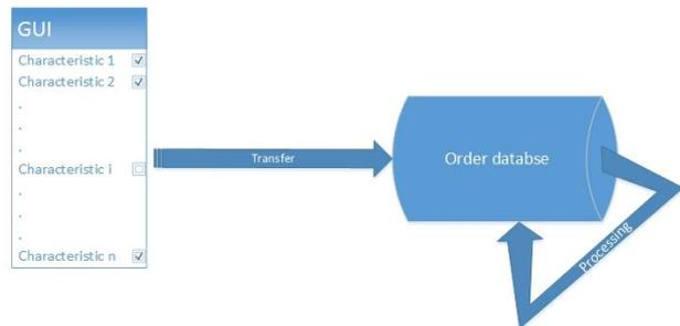
Fig. 5 – Order registration and processing in a smart product manufacturing system
