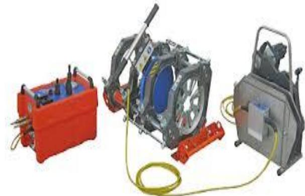
**Figure 3.** Machine for butt welding pipelines and fittings
