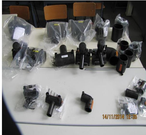
**Figure 4.** Fittings required for electrofusion and butt welding
